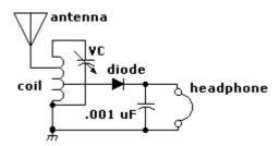
A coil, Variable capacitor to tune frequency, a crystal Diode and a High Impedance headphone, makes a crystal radio. You require a very good antenna and good ground. The .001uf Capacitor is to remove radio frequency from the signal.
